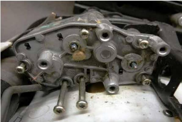
1. Raise seat to its highest position before starting. At this point you want to **disconnect the battery** so as not to turn on the SRS light when disconnection wiring. Remove seat from vehicle. There are two bolts on the front tracks of the seat, and two on the back. All four need to be removed. Then, disconnect the electrical wires connecting to the seat - three in my case. (NOTE: I found it easier to lift the seat off the bolts and tilt it sideways to get a better grip on these.)
