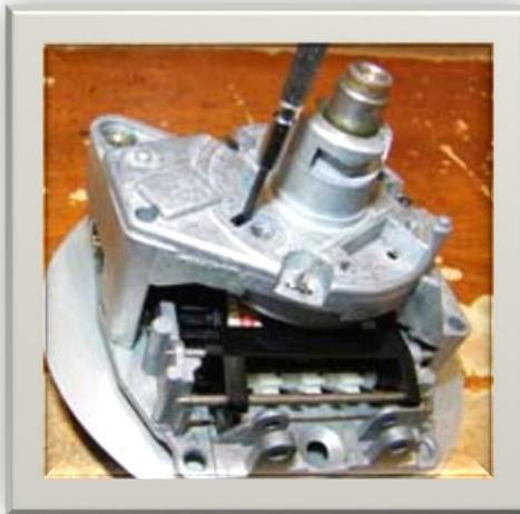
Insert a small slotted screwdriver (like the one shown) into one of the holes. This will lock the speed cup and mechanism inside the speedometer so the needle shaft cannot move.
