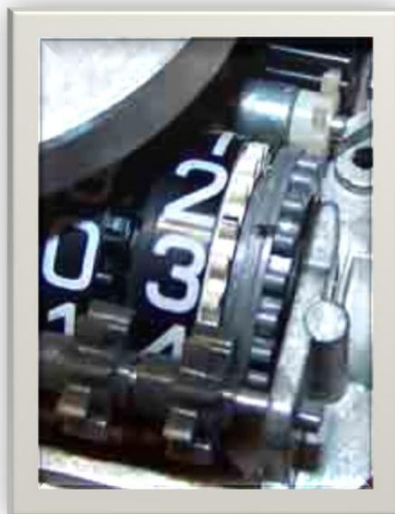
\*Then I used a felt marker and marked both the gray metal gear and the white plastic one next to it. I wanted the gray metal gear to go back in the exact **same position**, in case it made a difference.
