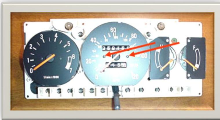
\* Once the needle is off, remove the metal speedometer faceplate using a small flat screwdriver to remove the 2 tiny screws.
