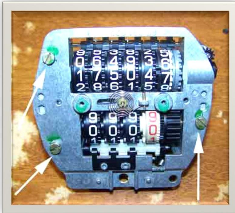
\*Here's the naked speedometer after removing the faceplate. See those 3 slotted screws? Remove them. They hold the two halves of the Speedo together. Once the screws are removed, be gentle when pulling in apart. The parts inside are delicate, but it won't explode... trust me. You'll see one piece that can fall out at this point, but not to worry, just put it back like the picture.
